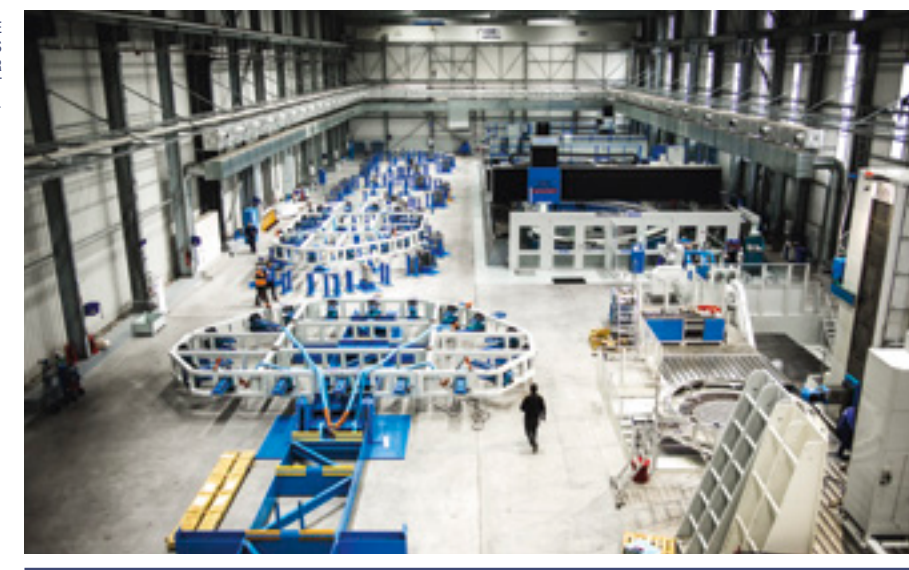
MANUFACTURE OF RADIAL PLATES FOR THE ITER PROJECT AT LA SEYNE-SUR-MER.
