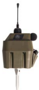
UMRA Mini - Seismic & acoustic detection and classification
