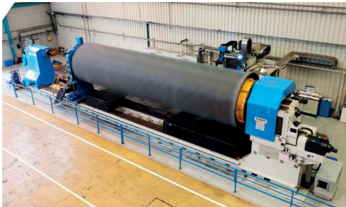
Tour horizontal (L 15000 mm, charge max. 40 tonnes).
