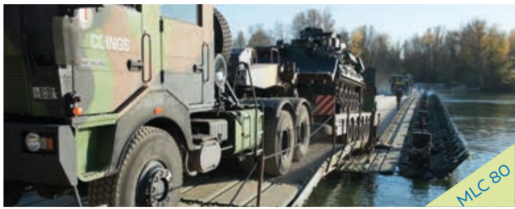
Loaded Leclerc tank carrier on 160m long bridge
