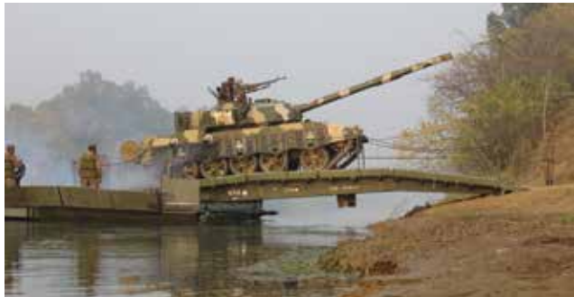
Multi purpose tactical ramp* : / no bank preparation / interoperability with other floating bridges / dry gap crossing * The multi purpose tactical ramp is also available for the PFM XP configuration
